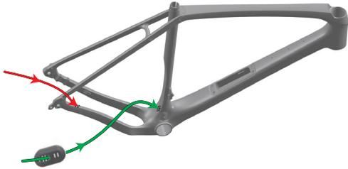
4. Connect the shift housings to the derailleurs. Insert the grommet (3) into the frame.
