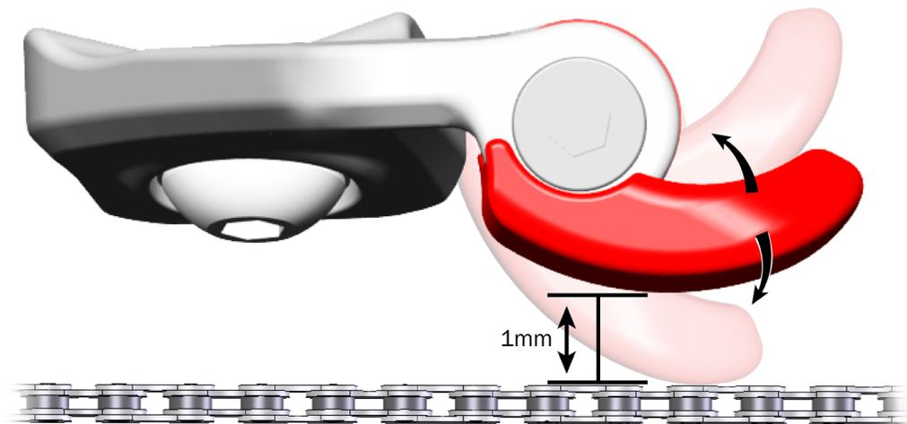
4. Tighten the bolt (1) to 1Nm.
