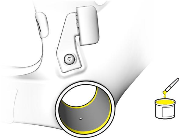
2. Using your hands, thread the bottom bracket onto the frame.
