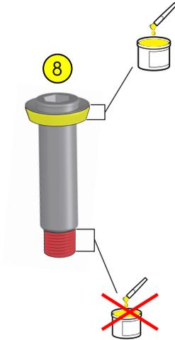
6. Install the hardware as shown on page 12. Torque the bolt (8) to 12.5Nm.
