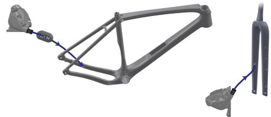
3. Attach the calipers to the chainstay and fork. Do not fully torque the mounting bolts until the calipers are aligned correctly.
