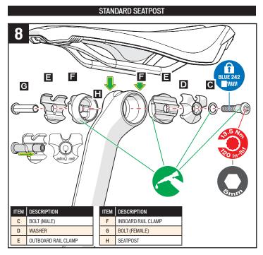
FIG.8: Install the saddle.
