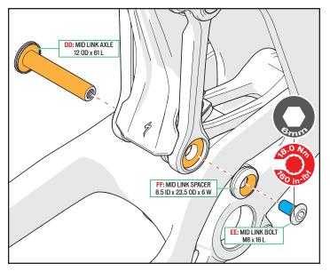
Grease, then insert the mid link axle DD into the non-drive side mid link, place the drive side bolt EE through the drive side spacer FF, then thread it into the mid link axle.
