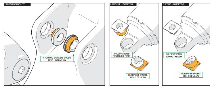
Grease, then install the forward shock eye spacers (x2) Y into the bearings.
