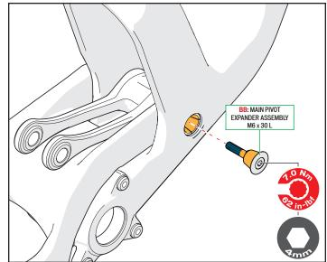
Grease, then thread the expander assembly BB into the main pivot axle and torque the bolt to 62 in-lbf / 7 Nm.
