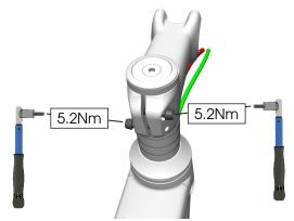
8. Install the faceplates and faceplate fasteners. Fully tighten the top two bolts before the bottom two (there will be a gap on the bottom).
