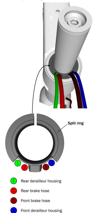
4. Route the bearing cover and shroud through the housings and snap them together. Make sure to press together any gaps.
