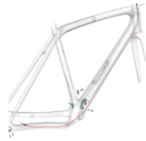
Brake/shift routing — mechanical
